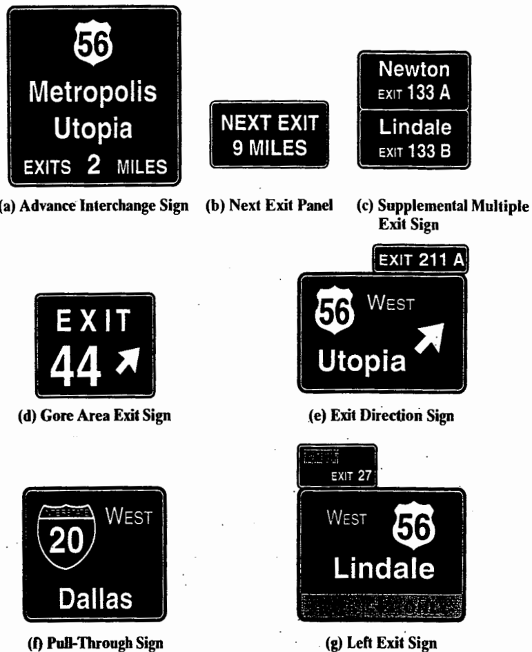
Figure 4.15: Sample Freeway and Expressway Destination Signs
